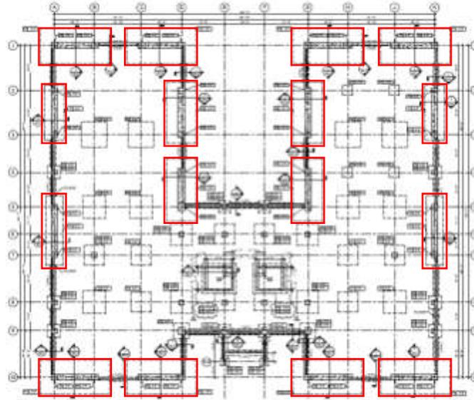
Figure 3: Braced Frames/Combined Footing Locations
