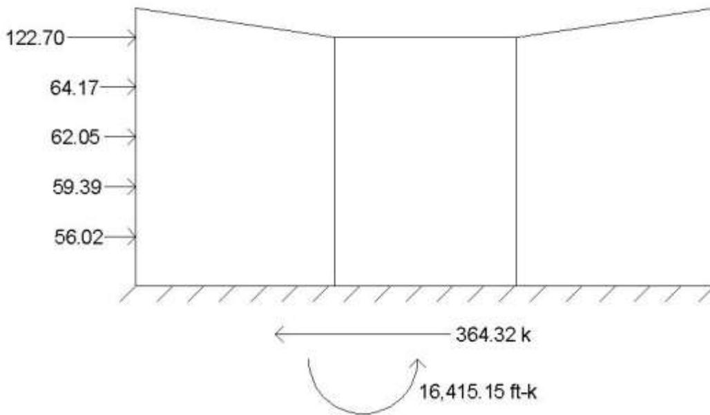
Figure 16: E-W Wind Force Diagram
