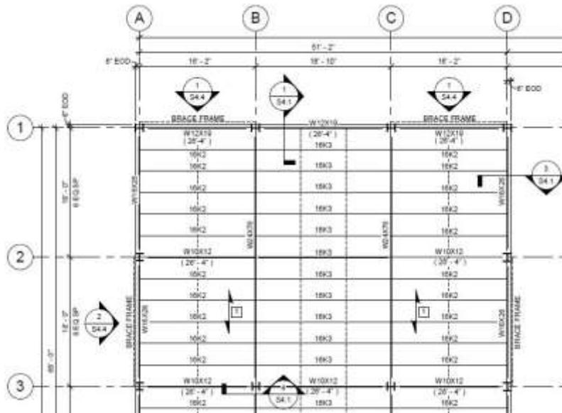
Figure 4: Typical Floor Framing Plan (Enlarged)
