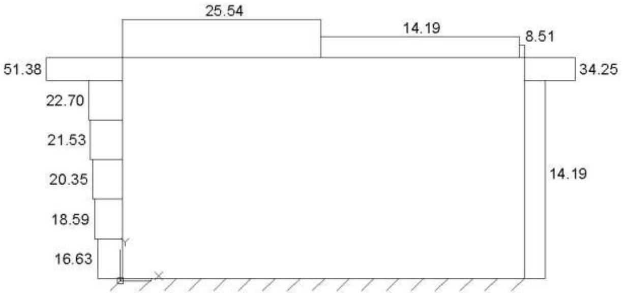
Figure 11: N-S Wind Pressure Diagram
