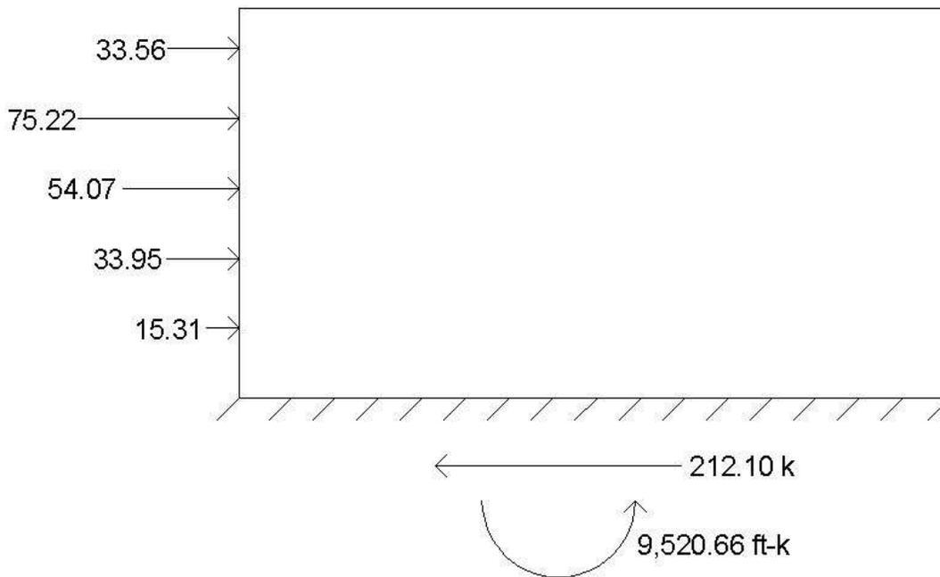
Figure 18: Seismic Force Diagram
