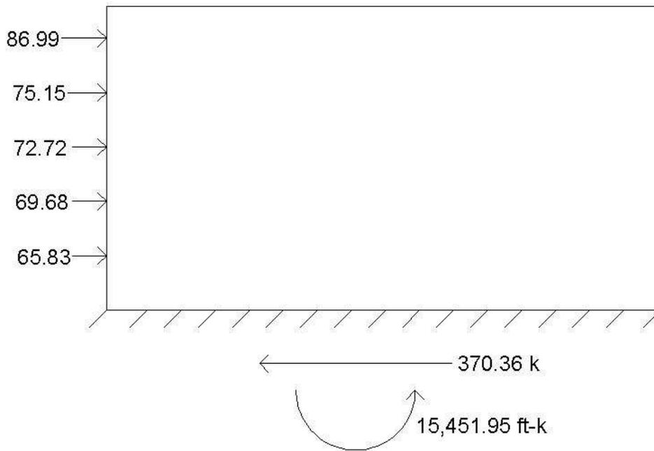
Figure 12: N-S Wind Force Diagram
