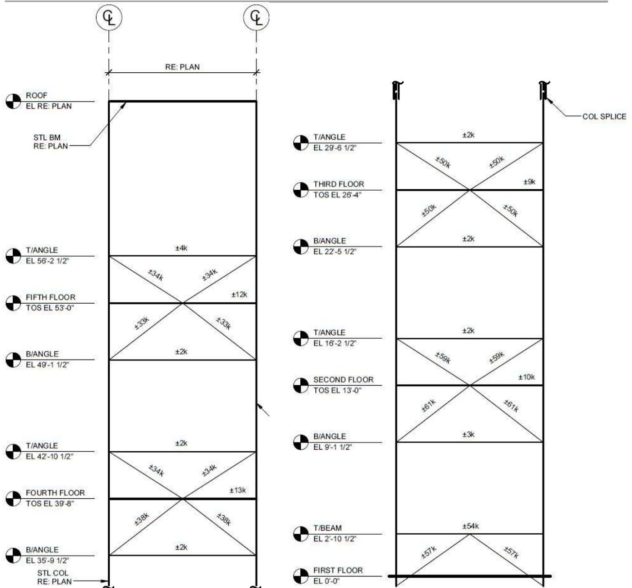
Figure 19: Typical Braced Frame and Bracing Details
